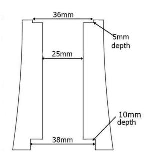
The mill should be assembled as in the diagram below.
